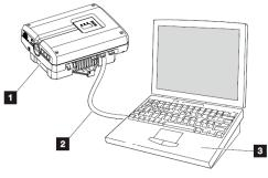
Fig. 52: Connecting inverter and computer with an Ethernet cable
